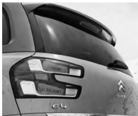
Figure 1 The plastic tailgate can be designed with uniquely shaped taillights
