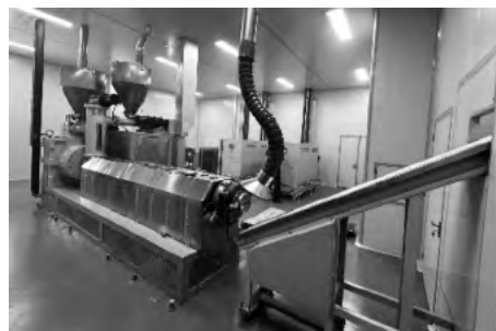
Figure 1 Medical PVC calendering single screw extrusion unit
