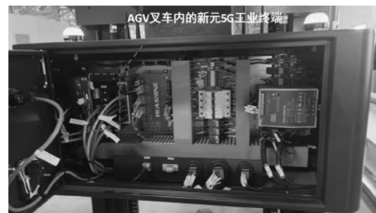
Figure 4 5G industrial terminal integrated into AGV forklift
