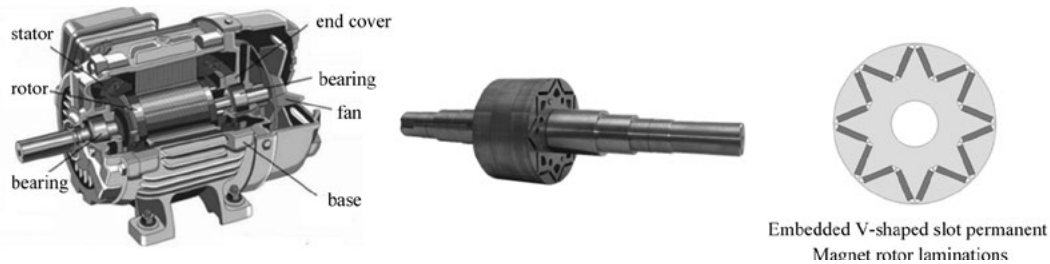
Figure 3 Composition of permanent magnet synchronous motor
