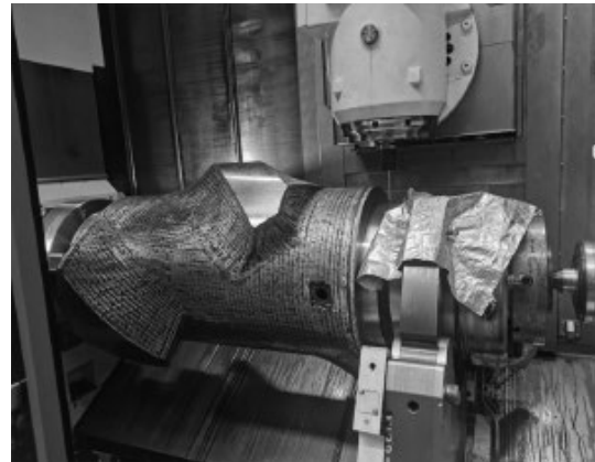
Figure 8 Actual photo of the protection site, showing the precision milling of the rotor body.
