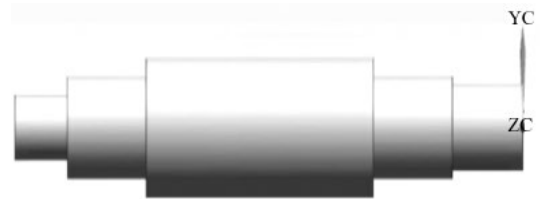
Figure 4 Semi-finished product after semi-finishing turning
